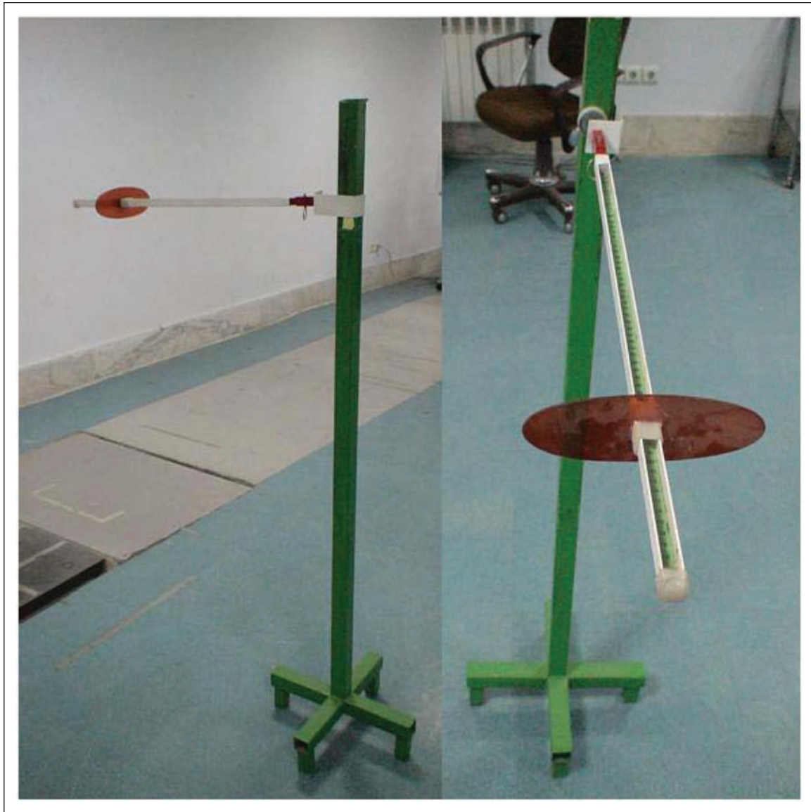
Figure 2. The front (right) and lateral (left) views of the device used for functional reach test.
