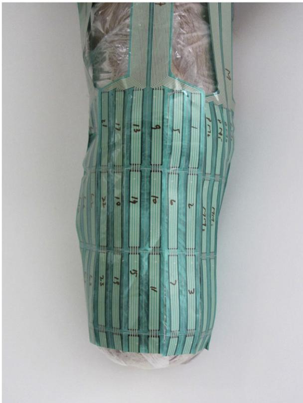
Fig. 1. Placement of sensors on residual limb.
